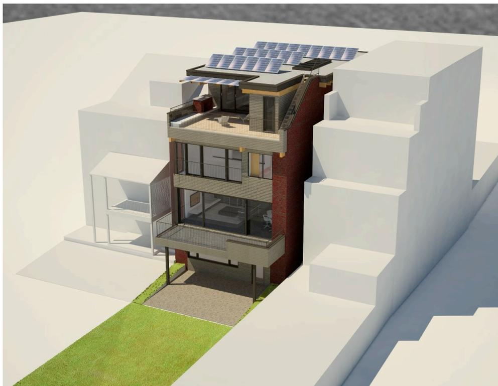
AVACOS SOLAR is pleased to announce the first Canadian residential photovoltaic system featuring a combination of the SANYO HIT (Heterojunction with Intrinsic Thin-Layer) Double Bifacial solar PV modules and the DuROCK Tio-Coat reflective 'cool' roof membrane coating.
